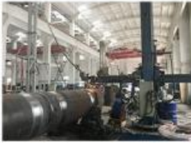
9. SUBMERGED ARC WELDING
