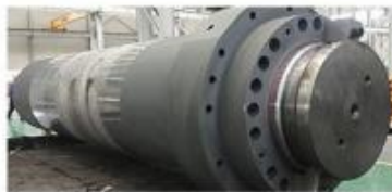
HYDRAULIC PRESS CYLINDER
