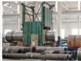
10. HEAT TREATMENT AFTER WELDING
