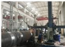
9. SUBMERGED ARC WELDING
